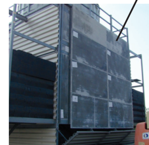
Series ES FireStop™ structural concrete liner installation for FM test
